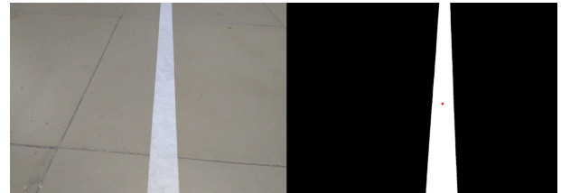
Fig. 11. A sample frame (left) and the processed frame (right) with the centroid in red.
